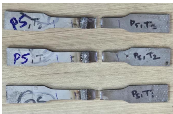
Fig 4: Fractured tensile sample
